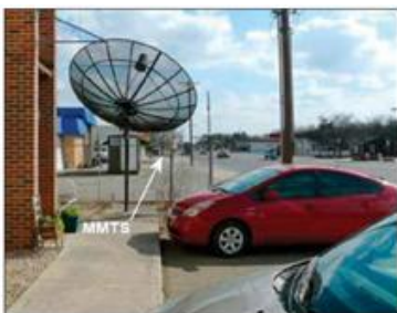
Figure 16. The recently moved temperature station in Lampasas, Texas - now in the parking lot of a downtown radio station.
